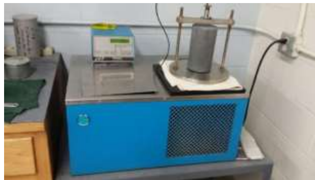
Figure 3-14 Coefficient of Thermal Expansion Testing Apparatus
