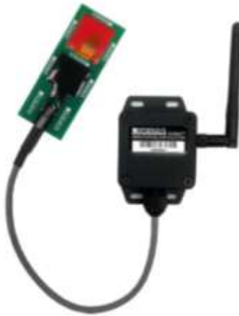
Figure 7-1 SenSpot -Strain Gauge (14)
