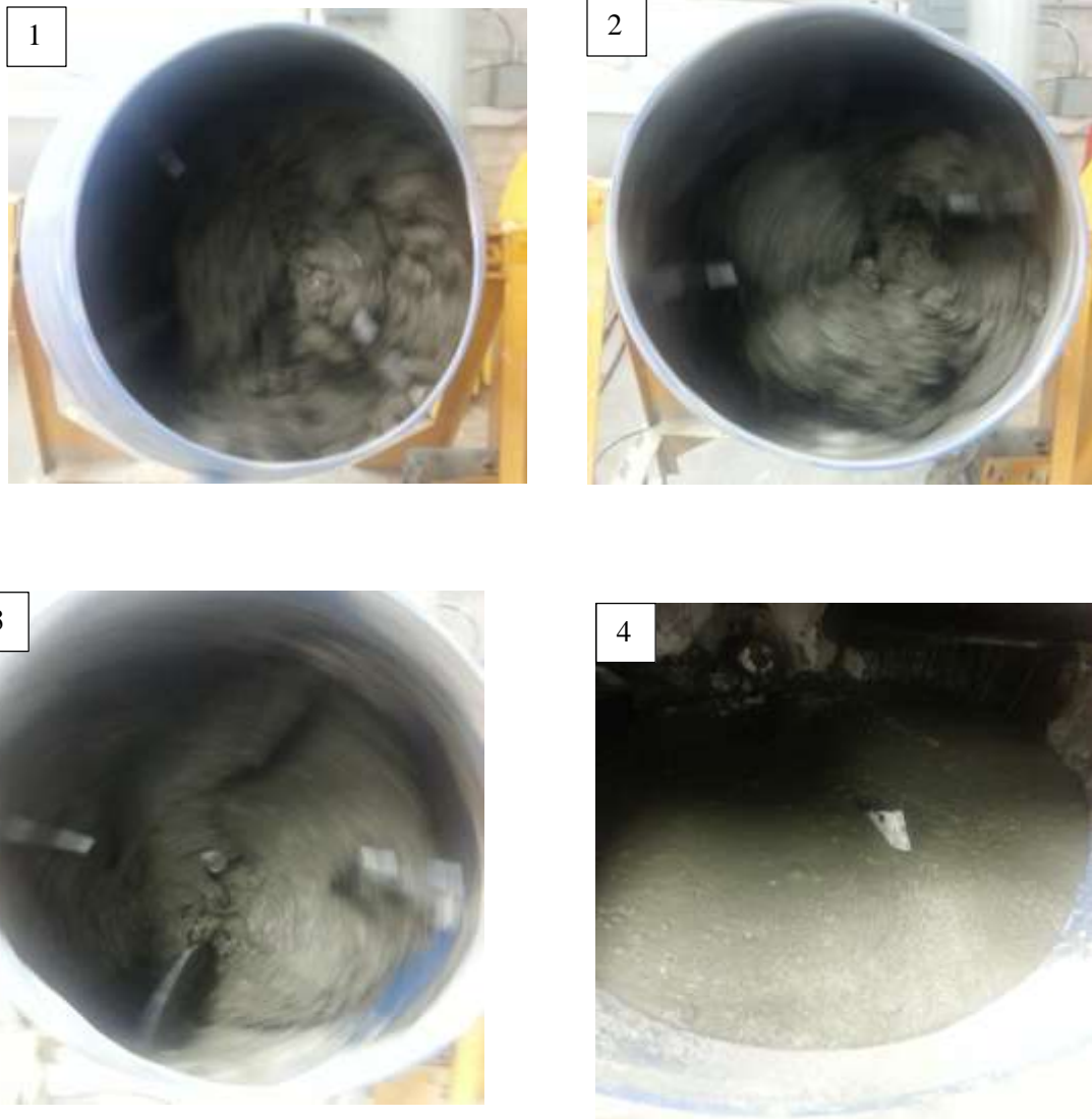
Figure 3-34 Mixing Process of 1.5 ft 3 of K-UHPC
