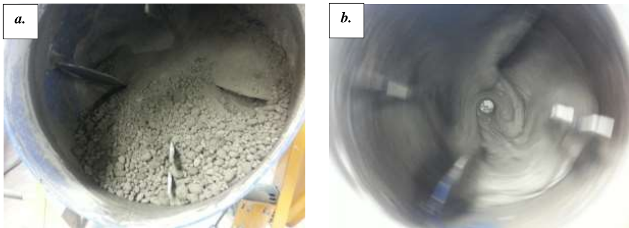
Figure 3-18 Mix 3 Condition after Liquid Additives a) Poor, b) Good
