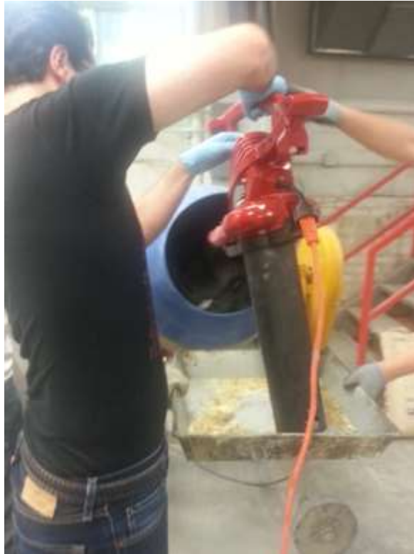
Figure 3-35 Adding Steel Fibers using a Blower
